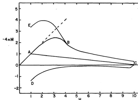
FIG. 2. Magnetization curve corresponding to  $\beta t = 12.5$ . Region ABC corresponds to Fig. 1(a), region CD to Fig. 1(b) and region EB to Fig. 1(c).
