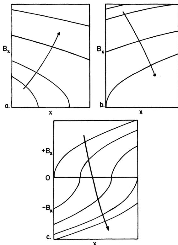
FIG. 1. Schematic indication of variation of fluxoid density (identical with  $B_x$ ) with position at various stages of the magnetization curve. (a) Arrow indicates increasing  $H$  (virgin specimen). (b) Arrow indicates decreasing  $H$ . (c) Arrow indicates increasing negative  $H$  (cyclic condition).
