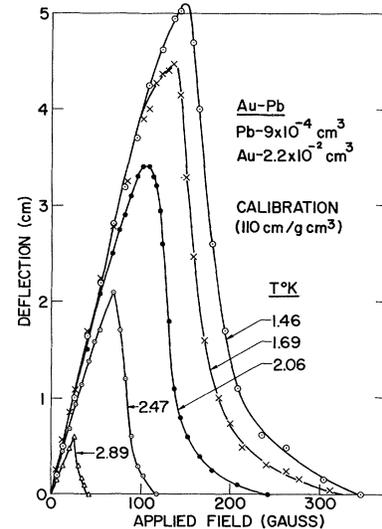
FIG. 3. Magnetic moment (calibration as shown).
