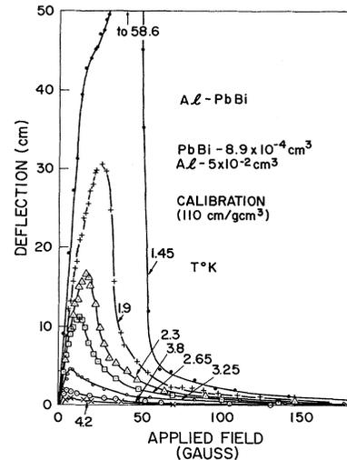
FIG. 2. Magnetic moment (calibration as shown) of Pb-Bi filaments in Al.
