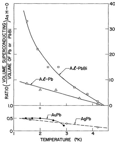
FIG. 1. Weak magnetic field susceptibility of composite wires. Filaments of Pb or PbBi are  $\sim 350 \text{ \AA}$  radius and shells are Al  $\sim 1400 \text{ \AA}$  surrounding Pb, Al  $\sim 300 \text{ \AA}$  surrounding PbBi, Ag and Au  $\sim 300 \text{ \AA}$ .
