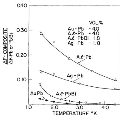
FIG. 4. Ratio of the free energy difference  $\Delta F$  of the composite to the free energy difference of the volume of Pb or PbBi as noted in the figure.
