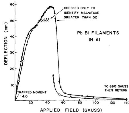
FIG. 9. Magnetization curve of PbBi filaments in aluminum.
