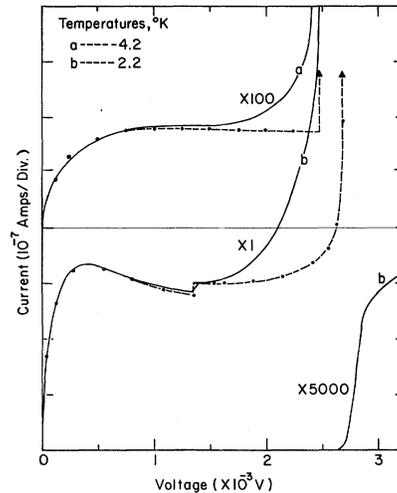
FIG. 1. Typical experimental I-V curves (solid lines) for Pb-Pb junctions. The dashed lines are theoretical SPT plus DPT I-V curves.
