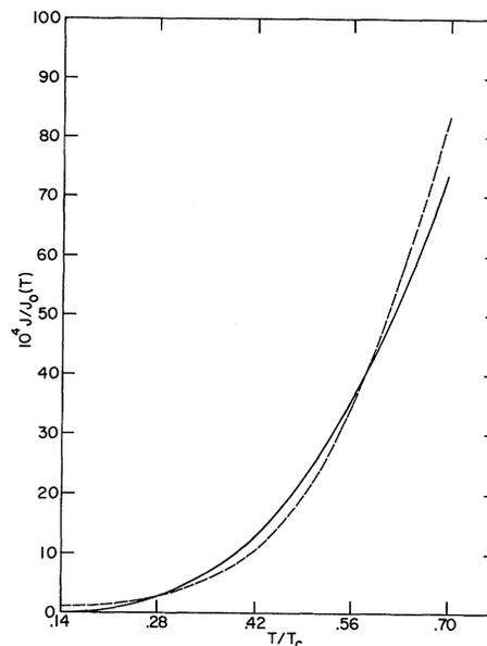
Fig. 4. Theoretical (solid line) and experimental (dashed line) plots of normalized current  $J/J_0(T)$  vs reduced temperature for  $eV/2\Delta(T) = 0.8$ .
