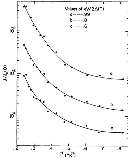
FIG. 2. Normalized excess current  $J/J_0(0)$  vs reciprocal temperature for several values of  $eV/2\Delta(T)$ .
