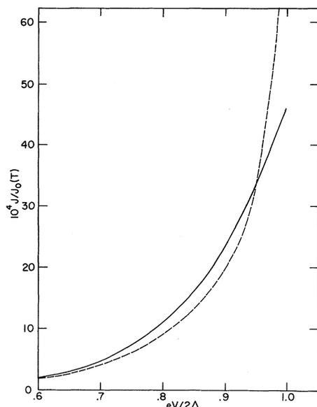
Fig. 3. Theoretical (solid line) and experimental (dashed line) plots of normalized current,  $J/J_0(T)$  vs voltage for  $T = 2.86^\circ\text{K}$ .
