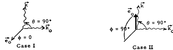
FIG. 2. Special cases of the scattering of a linearly polarized gamma ray.
