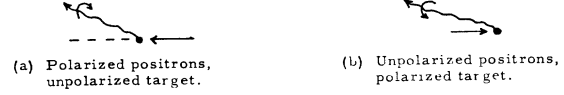
FIG. 18. Circular polarization produced by high-energy positron annihilation-in-flight when one of the particles is unpolarized. The electron target is on the left and the positron is incident from the right.
