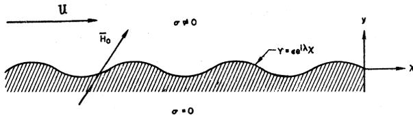
FIG. 1. Flow past a wavy wall where the applied magnetic field is uniform and oriented at an arbitrary angle with respect to the undisturbed free-stream velocity  $U$ .
