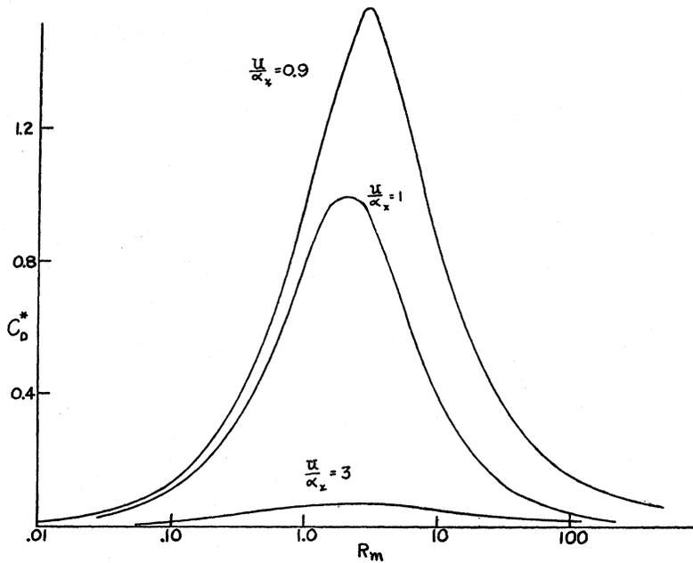
FIG. 3. Drag coefficient  $C_D^*$  plotted vs  $R_m = \sigma Ul$  for various values of the ratio  $U/\alpha_x$  for the case where  $U$  is aligned with  $H_0$ .
