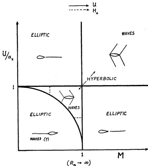
FIG. 5. Various flow regimes in the  $U/\alpha_x, M$  plane. The dotted lines refer to the curves plotted in Fig. 6.
