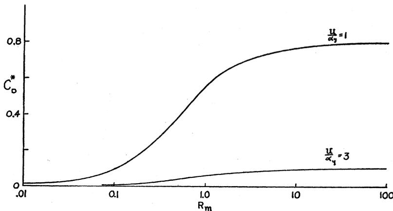
FIG. 4. Drag coefficient  $C_D^*$  plotted vs  $R_m = \sigma Ul$  for various values of the ratio  $U/\alpha_y$  for the case, where  $U$  is perpendicular to  $H_0$ .
