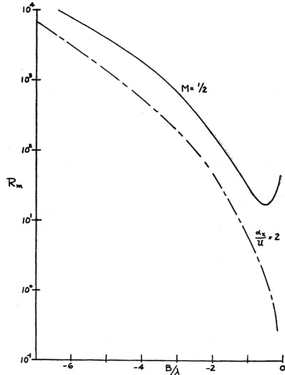
FIG. 6. The magnetic Reynolds number ( $R_m = \sigma Ul$ ) required for currents to damp to  $1/e$  of the wall value in a distance  $l$  along the waves vs the cotangent of the wave angle  $B/\lambda$ .
