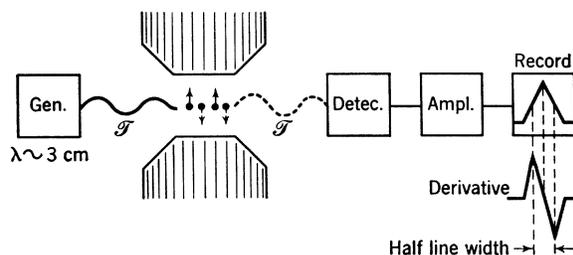
FIG. 2. Absorption of 3-cm waves resulting from transition of free electrons between energy states in an external magnetic field.
