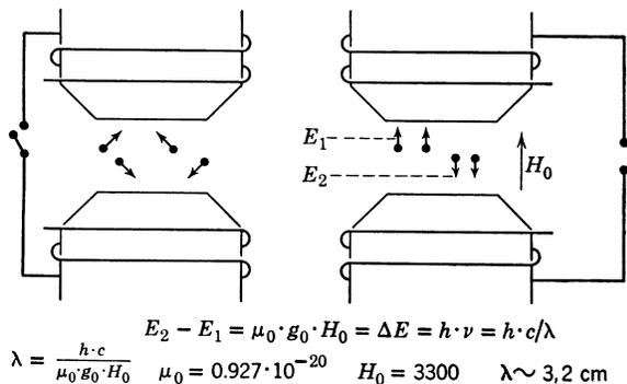
FIG. 1. Energy states of free electrons in an external magnetic field.
