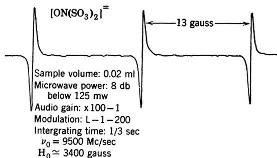
FIG. 3. ESR spectra of nitrosyl disulfonate [from Varian Associates Technical Information Bulletin, No. 2, 11 (1958)].
