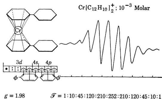
FIG. 5. Paramagnetic-resonance absorption spectrum of bisdibenzene chromium cation.
