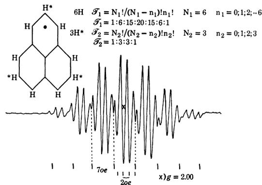
FIG. 6. Paramagnetic-resonance absorption spectrum of perinaphthényl radical.
