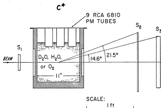
FIG. 1. A typical apparatus for measuring antiproton collision cross sections. The antiproton is certified by scintillator  $S_1$ , the box  $C^*$  contains the absorber, and the photomultiplier tubes recognize annihilation; scintillators  $S_2$  and  $S_3$  recognize antiproton which pass through.
