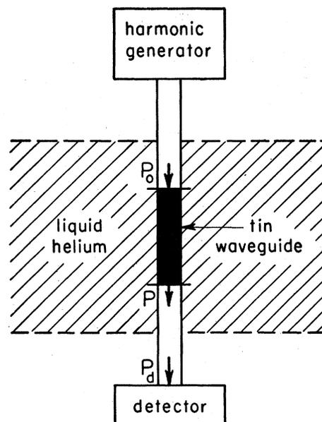
FIG. 19. Simplified diagram of apparatus used to determine the transmission of superconducting tin wave guide. The experiments of Blevins, Gordy, and Fairbank (Duke University group) and of Biondi, Forrester, and Garfunkel (BFG) are based on this method.
