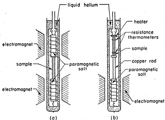
FIG. 2. Schematic diagrams of apparatuses for measurement of thermal conductivity below 1°K; (a) Goodman's rate of approach to equilibrium method, (b) steady-state method of Laredo and others.
