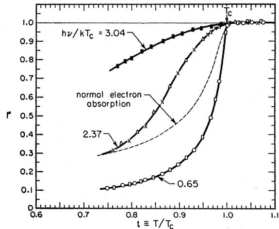
Fig. 22. Absolute measurements by BGM of the surface resistance ratio *vs* reduced temperature for bulk aluminum. The dashed curve represents the absorption by the normal electrons at  $h\nu = 2.37kT_c$  (see text).
