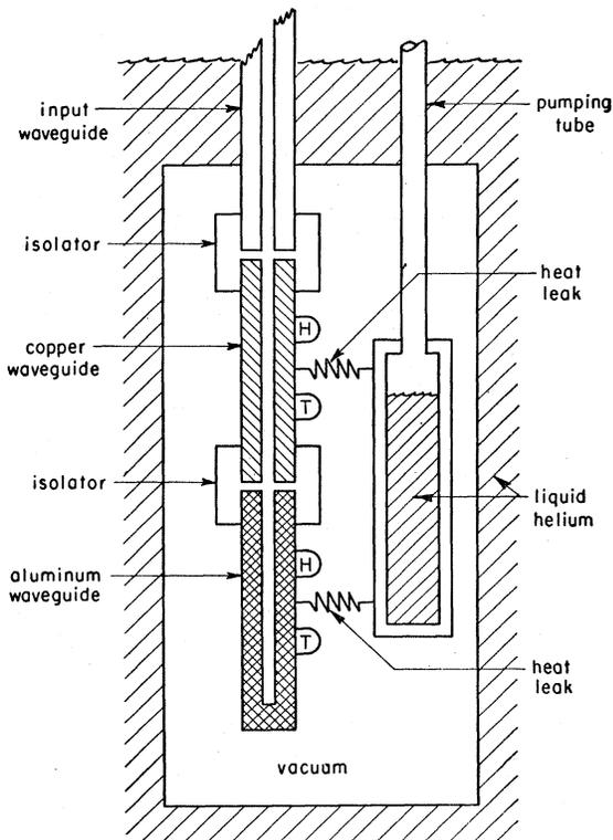
FIG. 20. Simplified diagram of the apparatus of Biondi, Garfunkel, and McCoubrey (BGM) used to measure the absorptivity of superconducting aluminum wave guide. The symbols  $H$  and  $T$  refer to heaters and thermometers, respectively, which are attached to the samples.
