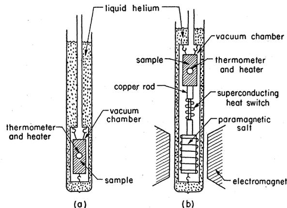
Fig. 4. Schematic diagrams of specific heat apparatuses; (a) for use in the liquid helium region, 1–5°K, and (b) for use below 1°K.
