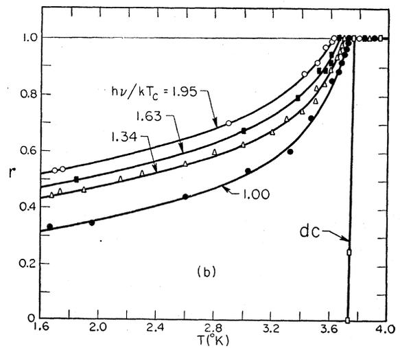
FIG. 21. Measurements by the Duke University group of the surface resistance ratio,  $r$ , as a function of temperature; (a) absolute determinations from  $Q$  measurements on a tin-plated cavity, and (b) measurements obtained from transmission data for tin-plated wave guide. In (b) the zero of the scale is determined by comparison with the cavity data.
