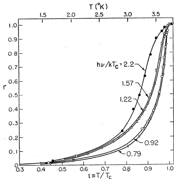
FIG. 23. Measurements by BFG of the surface resistance ratio for extruded tin wave guide. The curves are fitted so that  $r(T) \rightarrow 0$  as  $T \rightarrow 0$ .
