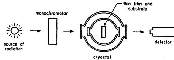
Fig. 25. Schematic representation of apparatus for measuring the transmission by a thin superconducting film.
