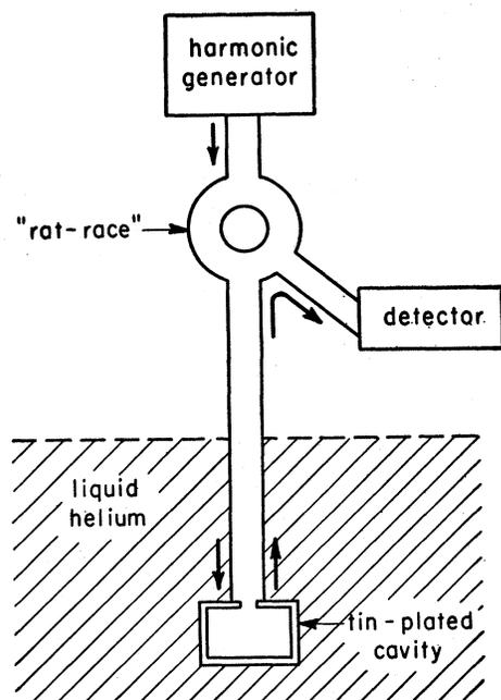
FIG. 18. Schematic diagram of apparatus of Blevins, Gordy, and Fairbank (Duke University group) used to determine the  $Q$  of a tin-plated cavity. The "rat-race" is a device which transmits power from the generator to the cavity and the reflected power from the cavity to the detector.
