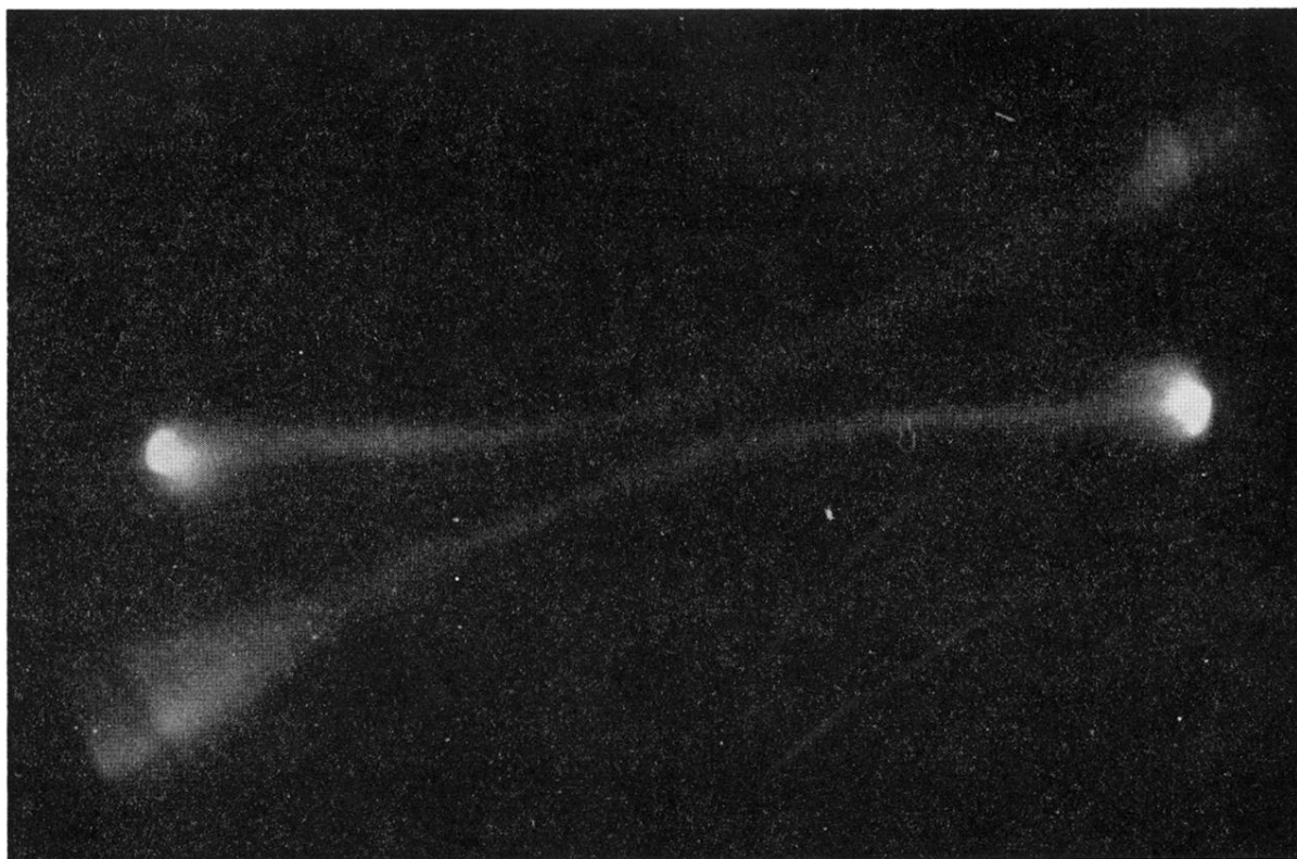
FIG. 1. Trajectories of plasmoids fired simultaneously at one another across a magnetic field of 4000 gauss at a pressure of 10^{-8} mm Hg with a separation distance of 10 cm.
