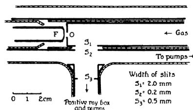
Fig. 5. Method II. Differential pumping. Special precautions to avoid thermal dissociation. (Smyth and Stueckelberg.)
