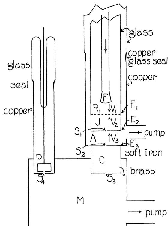
Fig. 3. Method II. Differential pumping. (Smyth).
