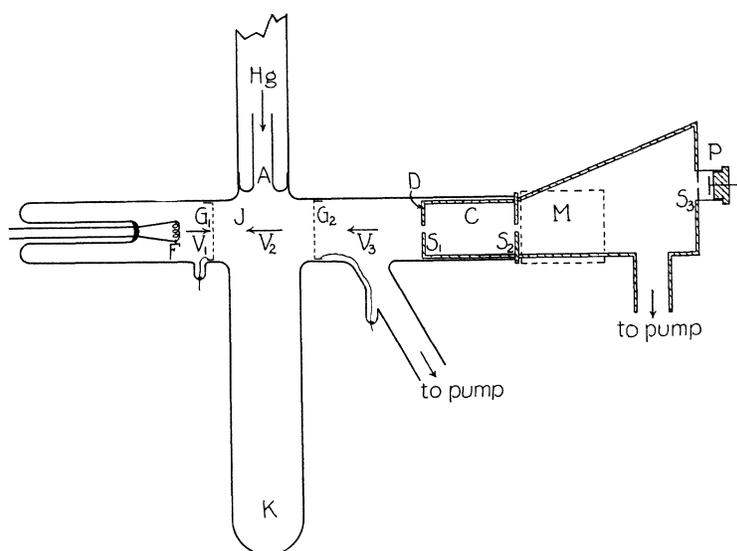
Fig. 2. Method I. Unidirectional vapor stream. (Smyth).
