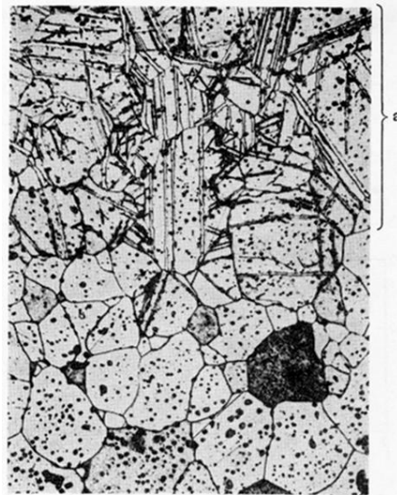
FIG. 5.11. Highly resistive surface layer (a) of manganese-zinc ferrite.
