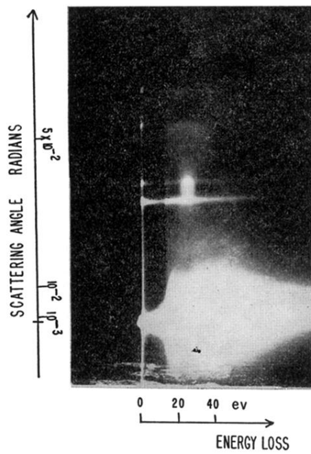
FIG. 10. Photographic record of energy loss vs angle as observed by Watanabe. 42 Angle is the ordinate and energy loss the abscissa. The characteristic loss at \sim 15 ev shows an arc-like variation of its energy value with angle (courtesy Dr. H. Watanabe).
