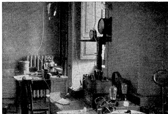
FIG. 2. The Geiger-Müller counter and lead houses used in the first year of the neutron work.
