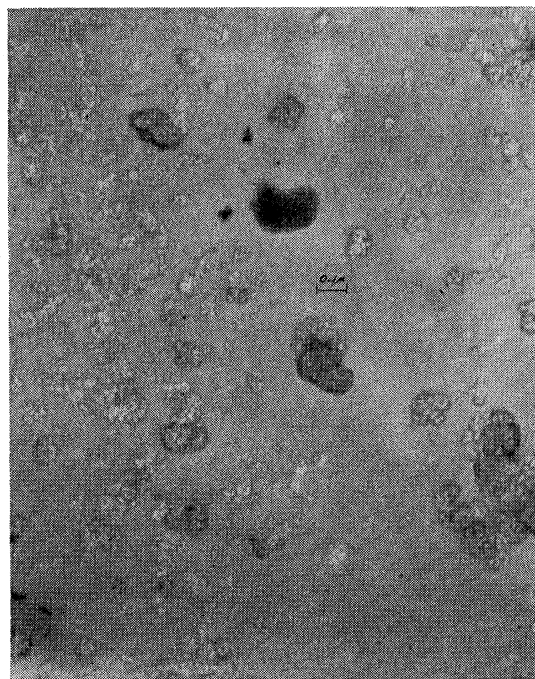
FIG. 3. Electron micrograph of same area as Fig. 2 after dissolving the iron particles to form a cavity. Some particles that have not been dissolved can be used as size reference.
