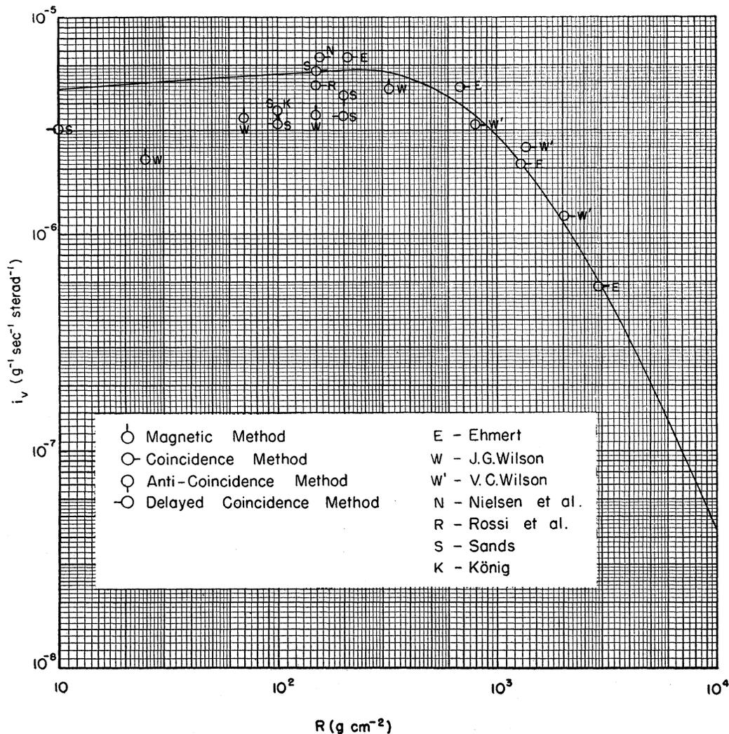
FIG. 6. Differential range spectrum of mesons at sea level. The range is measured in  $\text{g cm}^{-2}$  of air. The circles represent experimental data obtained by the following authors: Ehmert (E1), Koenig (K1), Nielsen *et al.* (N2), Rossi *et al.* (R4), Sands (S3), J. G. Wilson (W7), V. C. Wilson (W8).
