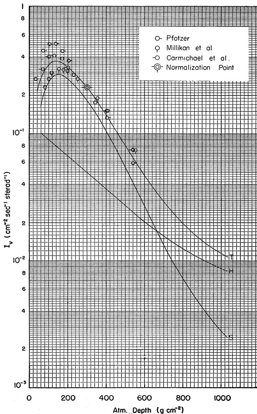
FIG. 2. The vertical intensities of the hard component ( $H$ ), of the soft component ( $S$ ), and of the total corpuscular radiation ( $T$ ) as a function of atmospheric depth at geomagnetic latitudes greater than  $45^\circ$ . Minimum range of the soft particles:  $5 \text{ g cm}^{-2}$  of brass.
