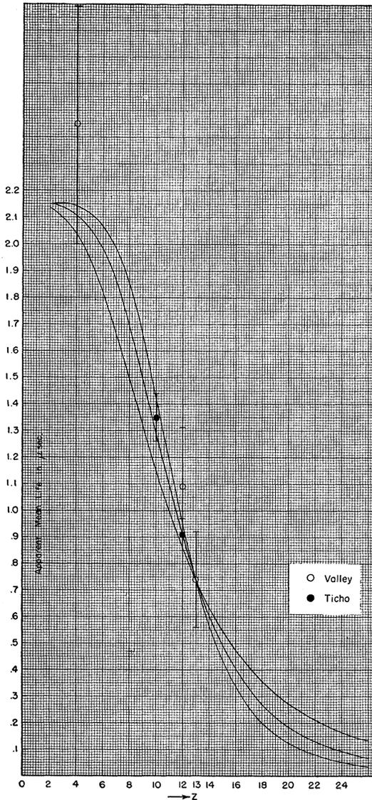
FIG. 8. Apparent lifetime of negative mesons as a function of the atomic number of the absorber. The experimental points were obtained with beryllium ( $Z=4$ ), sodium fluoride ( $Z_{Av}=10$ ), magnesium ( $Z=12$ ), aluminum ( $Z=13$ ). The three curves were computed under the assumptions that  $\tau_0$  is proportional to  $Z^{-3}$ ,  $Z^{-4}$ ,  $Z^{-5}$ , respectively, and were normalized to the experimental value for aluminum at  $Z=13$ .
