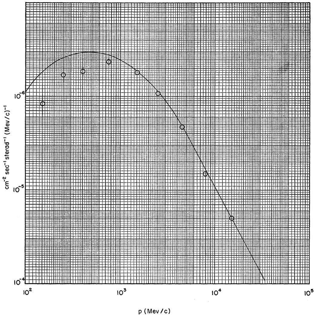
FIG. 4. Differential momentum spectrum of mesons at sea level. The circles represent experimental determinations by Wilson (W7). (Note: In the ordinate scale  $10^{-4}$  and  $10^{-5}$  should read  $10^{-8}$  and  $10^{-7}$ , respectively.)
