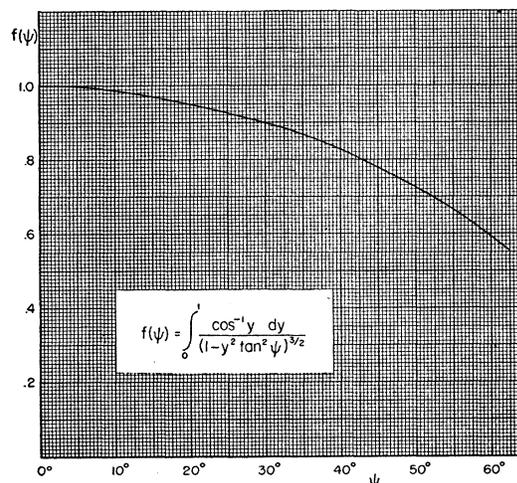
FIG. 26. Plot of the function  $f(\psi)$ . The quantity  $\tan\psi f(\psi)/\pi$  represents the fractional number of secondary particles projected away from the earth, under the assumption that these particles are produced with an angular divergence  $\psi$  by a primary radiation distributed isotropically in the upper hemisphere.
