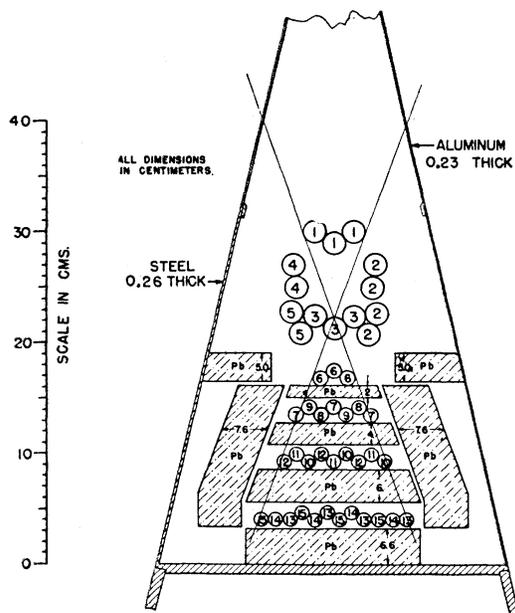
FIG. 13. Arrangement of G-M counters in the warhead of a rocket (from Golian and Krause G2).
