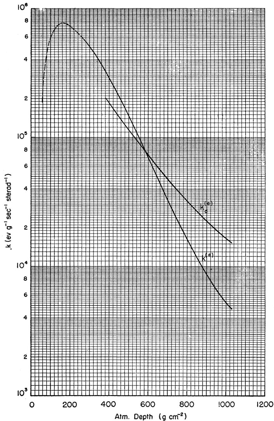
FIG. 19. The curve marked  $k^{(e)}$  gives the energy loss in the atmosphere of cosmic-ray electrons (exclusive of collision electrons). The curve marked  $k_d^{(e)}$  gives the energy loss of electrons arising from the decay of mesons, computed under the assumption that the whole energy set free by the decay goes into the electronic component.
