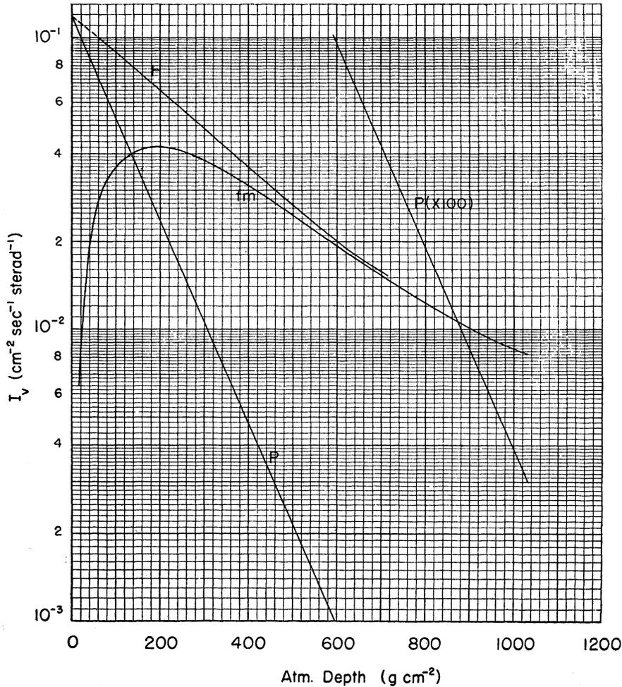
FIG. 16. Analysis of the hard component. The curve marked "fm" gives the vertical intensity of mesons with range greater than  $167 \text{ g cm}^{-2}$  of lead ("fast mesons"). The curve marked  $P$  represents the contribution of  $N$ -rays (high energy protons?) to the measured intensity of the hard component, but does not give an absolute value for the vertical intensity of these rays.
