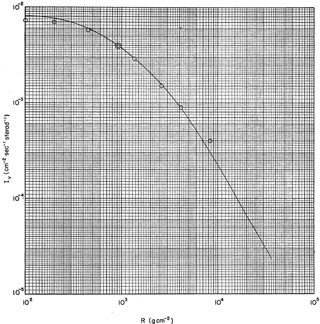
FIG. 5. Integral range spectrum of mesons at sea level. The range is measured in  $\text{g cm}^{-2}$  of air. The circles represent data obtained from the measurement of the momentum spectrum (W7), normalized at  $R=920 \text{ g cm}^{-2}$  (double circle).
