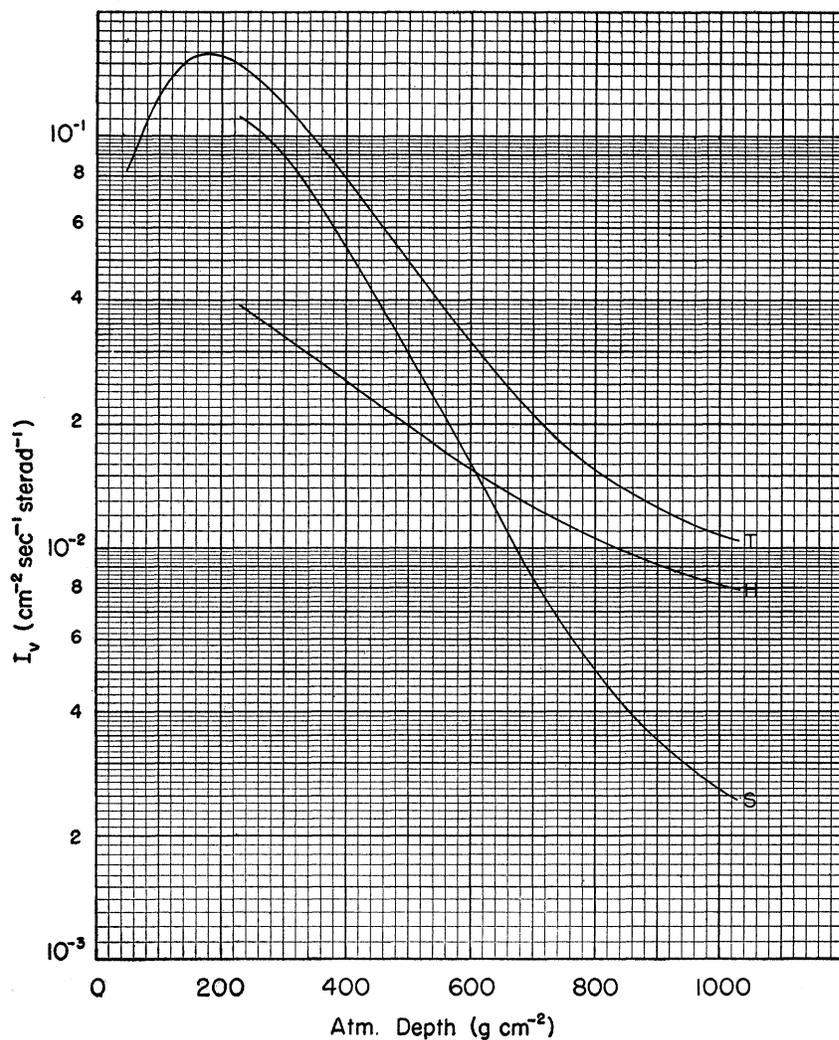
FIG. 3. The vertical intensities of the hard component ( $H$ ), of the soft component ( $S$ ), and of the total corpuscular radiation as a function of atmospheric depth near the geomagnetic equator. Minimum range of the soft particles:  $5 \text{ g cm}^{-2}$  of brass.
