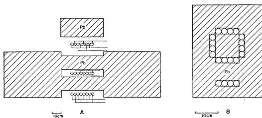
FIG. 11. Two experimental arrangements for the study of hard showers. *A* (J3): a record is obtained whenever one counter in each of the seven groups shown in the diagram is discharged. *B* (T6): a record is obtained whenever any two counters in each of the three horizontal trays is discharged. (The two vertical trays shown in the figure can be used to provide supplementary information on the structure of the showers.)
