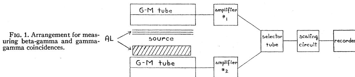
FIG. 1. Arrangement for measuring beta-gamma and gamma-gamma coincidences.
