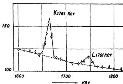
FIG. 12. Conversion peak of electrons from the  $K$ - and  $L$ -shells of the atom generated by  $\gamma$ -rays of 1761-keV energy. Comparison of the areas of the  $K$  and  $L$  peaks shows that the ratio of the probability of conversion on the  $K$ -shell to the probability of conversion on the  $L$ -shell equals 4.3:1.
