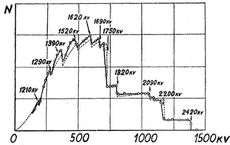
FIG. 5. Spectrum of internal conversion positrons of  $\gamma$ -rays from RaC. The abscissae give the energy of the positrons in keV, the ordinates, the number of positrons. The values given near the drops denote the energy of the corresponding  $\gamma$ -line in keV. The theoretical positron spectrum is shown by the dotted line.
