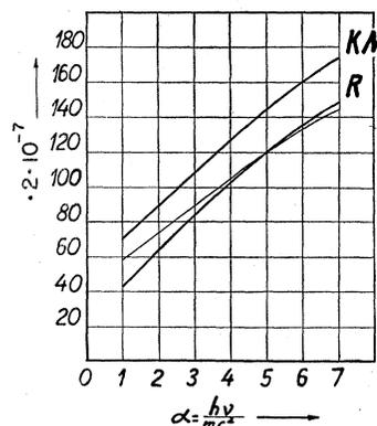
FIG. 4. The abscissae give the energy of the  $\gamma$ -quanta in  $mc^2$ ; the ordinates, the number of recoil electrons registered by the counters from each  $\gamma$ -quantum striking the target  $M$  (see Fig. 1). The curve  $R$  takes into consideration both the spectral distribution of the recoil electrons depending on the energy of the  $\gamma$ -quanta and the scattering of the Compton electrons in the target. The curve  $R$  is computed for the magnetic spectrograph shown in Fig. 1.
