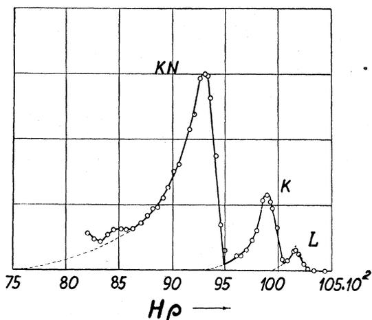
FIG. 17. Spectrum of Compton and photoelectrons generated in a lead lamina upon the passage through it of 2620-keV  $\gamma$ -rays. Peak  $KN$  corresponds to recoil electrons, peaks  $K$  and  $L$ —to photoelectrons from the  $K$ - and  $L$ -shells of the lead atoms. The spectrum was recorded with the apparatus depicted in Fig. 1.
