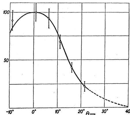
FIG. 21. Angular distribution of the photoelectrons. The points are plotted from the data of Fig. 20.
