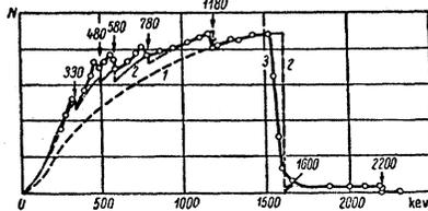
FIG. 6. Spectrum of internal conversion positrons of  $\gamma$ -rays from Th(C+C'). (See explanation to Fig. 5.)
