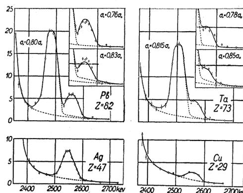
FIG. 18. Results of measurements of the photo-effect from the 2620-keV  $\gamma$ -line in Pb, Ta, Ag, and Cu. The dotted lines on the curves for Pb and Ta separate the photoelectrons generated in the  $K$ - and  $L$ -shells of the atom. The upper right-hand corner of the drawing shows how the curve would lie with respect to the experimental points if the two limiting values of the ratio  $\sigma_K/\sigma_a$  were taken.
