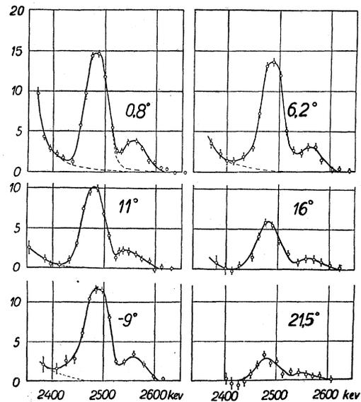
FIG. 20. Curves of photoelectrons, emerging from a lead lamina at different angles to the initial direction of the  $\gamma$ -quanta.
