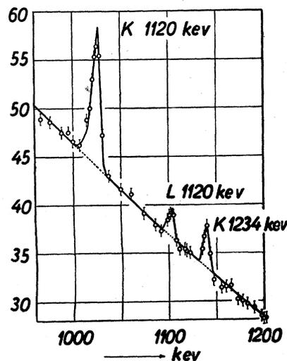
FIG. 14. Conversion peaks of electrons:  $K1120$  keV,  $L1120$  keV, and  $K1234$  keV. Comparison of the areas of the peaks  $K1120$  keV and  $L1120$  keV shows that the ratio of the probability of conversion on the  $K$ -shell to the probability of conversion on the  $L$ -shell equals 5.2:1.
