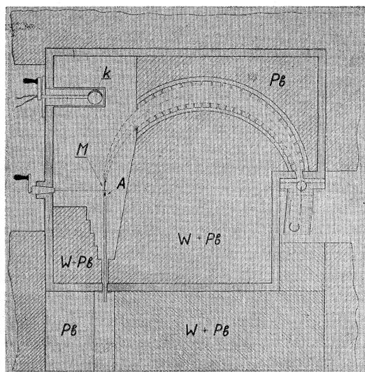
FIG. 1. Diagram of magnetic spectrograph. Cross section in the plane perpendicular to the magnetic field. *A*—radioactive source; *M*—target; *K*—coil for measuring the magnetic field; *W+Pb*—tungsten screen to shield the counter from the  $\gamma$ -rays of the source.
