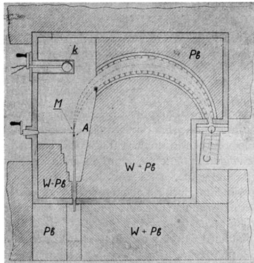
FIG. 1. Diagram of magnetic spectrograph. Cross section in the plane perpendicular to the magnetic field. *A*—radioactive source; *M*—target; *K*—coil for measuring the magnetic field; *W+Pb*—tungsten screen to shield the counter from the  $\gamma$ -rays of the source.
