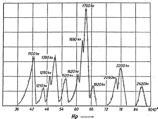
FIG. 2. Recoil electron spectrum of  $\gamma$ -rays from RaC. The abscissae give the energy  $H\rho$  of the recoil electrons; the ordinates—the number of electrons. The area of each peak is proportional to the number of recoil electrons generated by the  $\gamma$ -quanta of the given  $\gamma$ -line. The value of the energy of the  $\gamma$ -line in kv is denoted by the number near each peak. The vertical dashes indicate the statistical accuracy of the experimental points.
