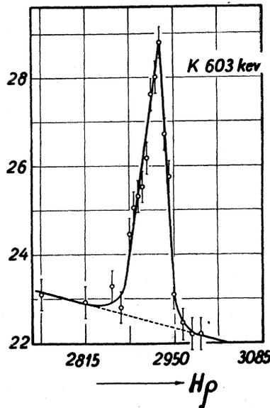
FIG. 15. Conversion peak of electrons generated in the  $K$ -shell of the atom by  $\gamma$ -rays of 603-kev energy.
