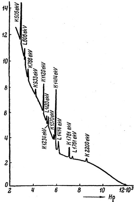
FIG. 9. Natural  $\beta$ -spectrum of RaC. The  $\beta$ -spectrum is given in the  $H\rho$  scale without recalculation for equal intervals of  $H\rho$ . The numbers near the conversion peaks denote the energy of the corresponding  $\gamma$ -line in kev. The letters  $K$ ,  $L$ , denote the electron shell of the atom where conversion of the  $\gamma$ -ray takes place.
