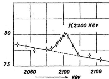
FIG. 11. Conversion peak of electrons from the  $K$ - and  $L$ -shells of the atom generated by  $\gamma$ -rays of 220-kev energy.
