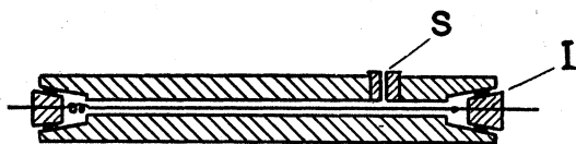
FIG. 17. Pirani-gauge of small volume. S, detector slit; I, insulator.
