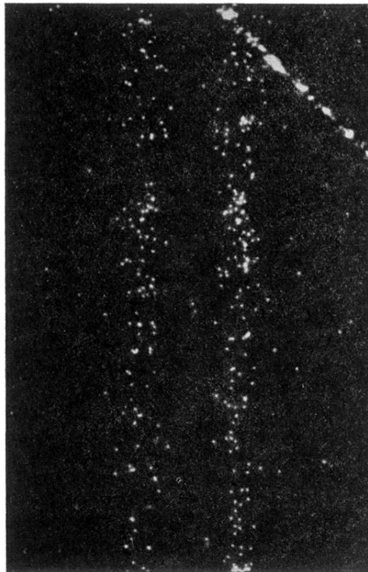
FIG. I-3. Difference in the action of positive and negative ions in producing condensation. The ions have diffused and formed into columns of positive and negative ions before the drops are formed. The denser column of drops is formed on positive ions. [From Hazen, Phys. Rev. 65, 259 (1944).]
