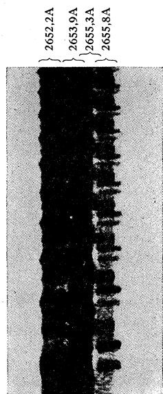
FIG. 2. Structure of the forbidden line \lambda 2655.8 ( 6^3P_0-6^1S_0 ) of mercury. A Fabry-Perot etalon was crossed with a large spectrograph. Exposure time 6 hours.
