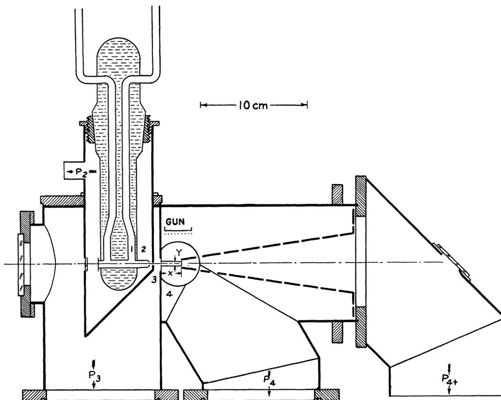
FIG. 3. Design of the apparatus described in Section IV. The "gun" is schematic. The heavy dashed line represents a removable funnel; cf. reference 32.
