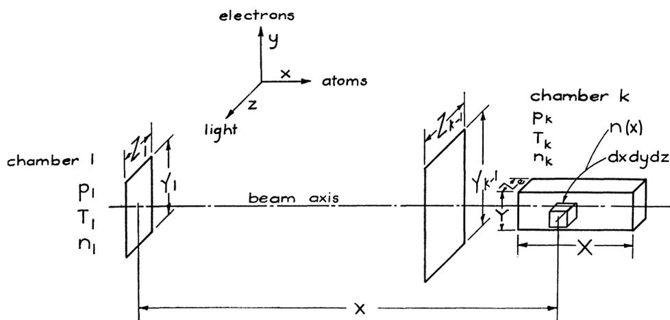
FIG. 1. Geometry of the atomic beam under discussion.
