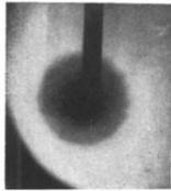
FIG. 58. Photograph of a low voltage arc in 0.05 mm A. The cylindrical cathode is viewed end-on and seen as a black circle with a thin bright edge; the figure shows the thin dark space-charge sheath and the relatively dark scattering sheath. The edge of the bulb may be seen in the left-hand bottom corner.
