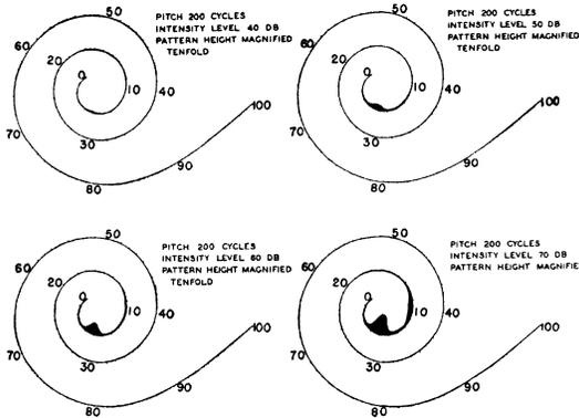
FIG. 7. Auditory patterns for a 200-cycle tone at various intensity levels.
