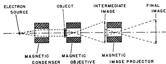
FIG. 22. Schematic diagram of magnetic type of electron microscope.
