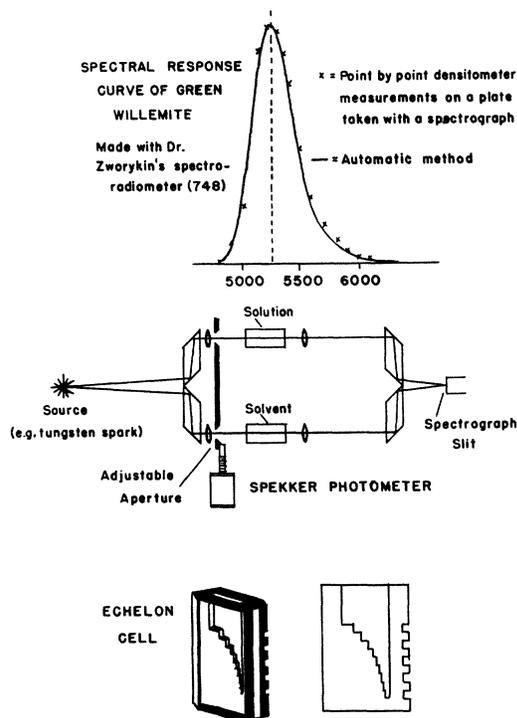
FIG. 6. Examples of spectrum methods and spectrophotometer apparatus.
