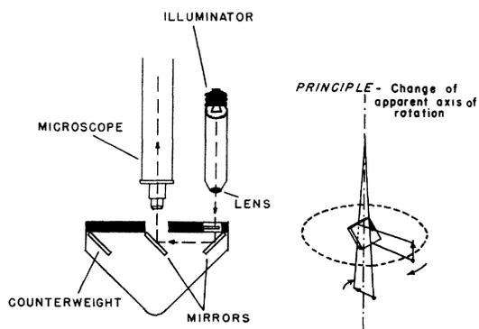
FIG. 18. Professor Harvey's centrifuge microscope, reference 992.
