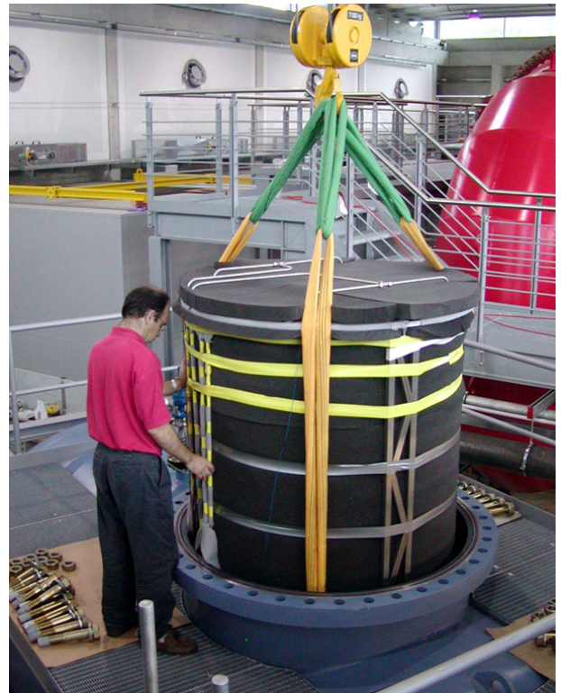
FIG. 4: The High-Pressure Convection Facility, weighing approximately 2000 kg, is being inserted into the turret of the “U-boat.”
