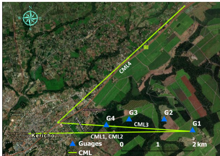
Commercial microwave links (straight lines) and rain gauges (triangles) near a farm in Kericho, Kenya.
