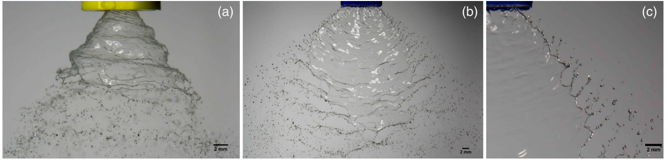
FIG. 1. (a) Picture of the conical nozzle with an operating pressure of 2.0 bar. The Squire wave is clearly visible, with a wavelength in agreement with the prediction. (b) The flat fan nozzle at 2.0 bar, with flapping and breakup occurring near the bottom of the picture. (c) Zoomed-in picture of the flat fan nozzle at low pressure (1.0 bar), showing droplets coming from the sheet's rim that are of the order of the nozzle size.
