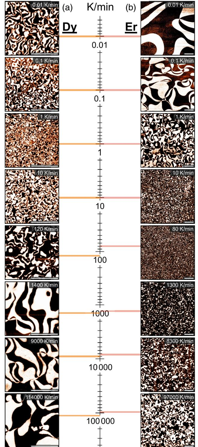
FIG. 2. Spatial maps of the vortexlike ferroelectric domain pattern in hexagonal manganites for a range of different cooling rates through  $T_c$ . Images were recorded by PFM under ambient conditions. Labels denote the respective cooling rates. Scale bar in all images is 5  $\mu\text{m}$ . (a) DyMnO<sub>3</sub>. (b) ErMnO<sub>3</sub>. The Kibble-Zurek-like increase of vortex density with cooling rate, followed by a reversal and decrease of vortex density, is clear in both compounds.
