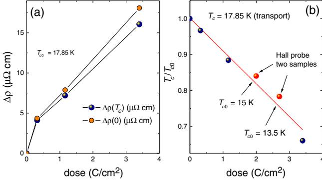
FIG. 2. (a) Change of resistivity of  $\text{Ba}(\text{Fe}_{1-x}\text{Ru}_x)_2\text{As}_2$  ( $x = 0.24$ ) at  $T_c$  and extrapolated to  $T = 0$  [see Fig. 1(b)] as a function of the irradiation dose. (b) Suppression of  $T_c$  with the dose of electron irradiation.
