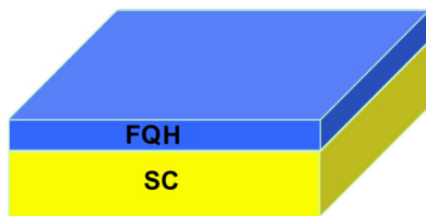
FIG. 1. Schematic setup of a fractional topological superconductor. This state of matter can be achieved by inducing a superconducting order parameter into a fractional quantum Hall bar or a fractional Chern insulator through the proximity effect.
