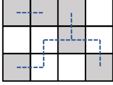
FIG. 7. A sample anyon configuration for noisy toric code. A dashed line on an edge denotes the corresponding qubit's phase is flipped by a Z operator. Anyons are created in plaquettes (shaded) where an odd number of dashed lines meet.
