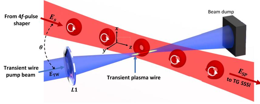
FIG. 4. Configuration for measuring the effect of a transient phase perturbation on field  $E_s$  (from a 4f-pulse shaper) imposed by the ultrafast OFI plasma induced by field  $E_{TW}$ . This OFI plasma is the transient wire. The perturbed pulse  $E_{sp}$  and unperturbed pulse  $E_s$  ( $E_{TW}$  off) are measured by TG-SSSI [17]. The angle between the beams is  $\theta = 18.5^\circ$ . A detailed experimental diagram is shown in Appendix C.
