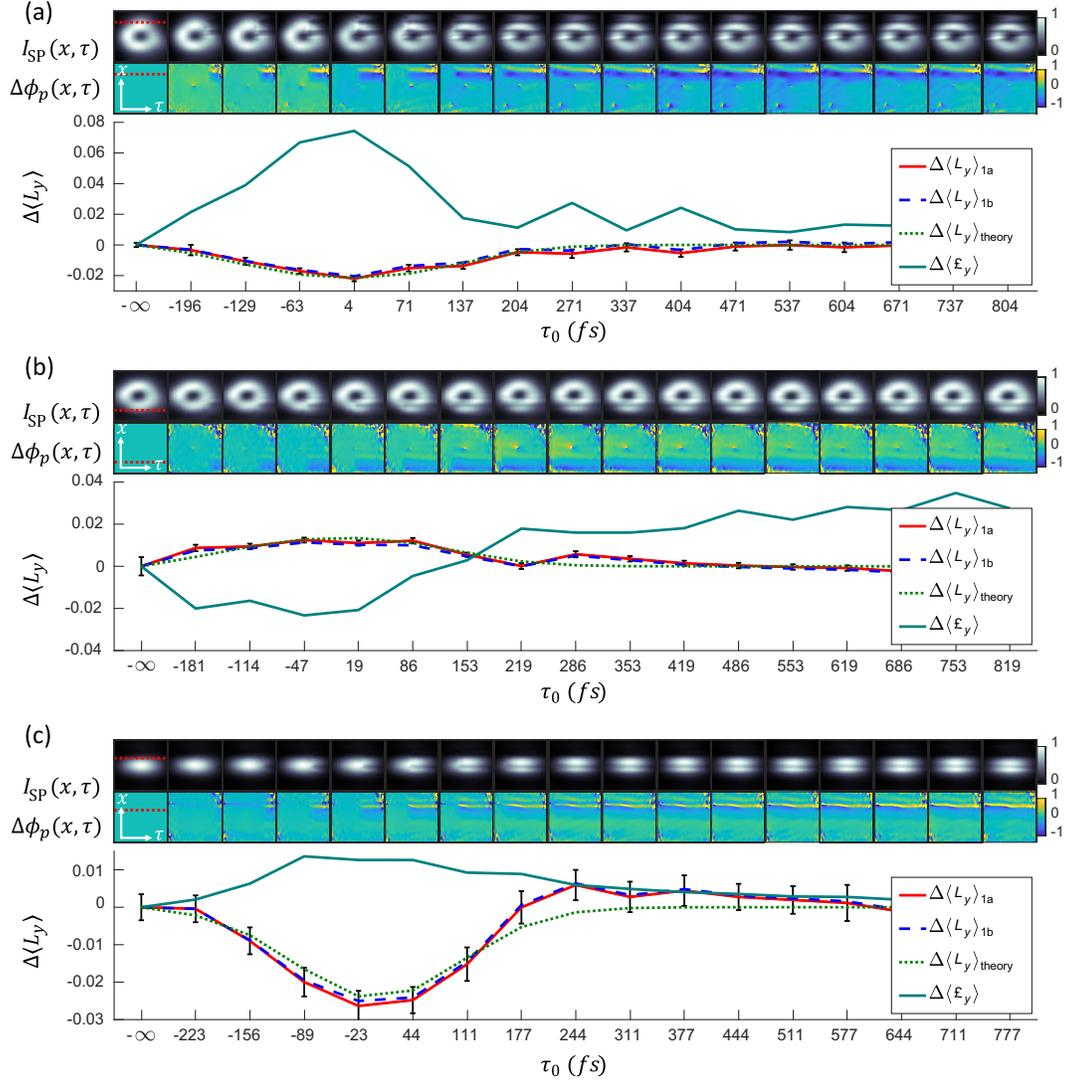
FIG. 9. Comparison of the predictions of Refs. [33,34] against our experimental results. The above panels replot the curves of Fig. 6 and overlay  $\Delta\langle\mathcal{L}_y\rangle$ , where the latter is computed using Eq. (1a), with the complex fields provided by the TG-SSSI measurements.
