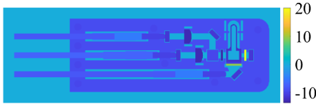
FIG. 13. Cross section of the 3D susceptibility model of the probe. The cross section is made through the center of the vapor cell. We cap the color scale at 20 ppm, even though the probe filter susceptibility is 140 ppm, to highlight the details of the entire structure.
