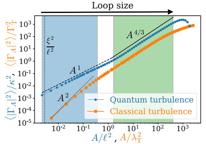
FIG. 2. Variance of the circulation around square loops of area  $A = r^2$ . The blue line shows the gGP simulation (resolution  $2048^3$ ), and the orange line shows the Navier-Stokes simulation (resolution  $1024^3$ ). The classical variance is rescaled by  $\Gamma_T^2 = (\lambda_T^4/3)\langle |\omega|^2 \rangle$ , with  $\lambda_T$  the Taylor microscale and  $\omega$  the vorticity field.
