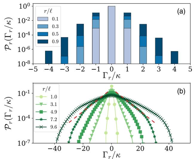
FIG. 3. PMF of the circulation in quantum turbulence for (a) loop sizes  $r/\ell < 1$  and (b) loop sizes  $r/\ell \geq 1$ . The red dashed lines are a guide for the eye indicating exponential tails. Note that all distributions are discrete, as  $\Gamma_r/\kappa$  only takes integer values. In panel (a), bars for  $\mathcal{P}_r(0)$  and  $r/\ell \geq 0.3$  are hidden behind the  $r/\ell = 0.1$  case. See Fig. 6 for details on  $\mathcal{P}_r(0)$ .
