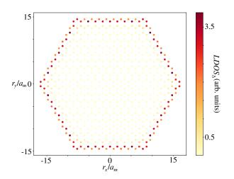
FIG. 3. In-gap local density of states in the QVH phase. We show the real-space plot of the local density of states integrated over 1.66 < E/W < 2.00, with U/W = 0.5. Here,  $r_{x,y}$  is the position of the lattice sites in units of the moiré lattice spacing,  $a_m$ . The result is computed with open boundary conditions and parameters as in Table I from Appendix C.
