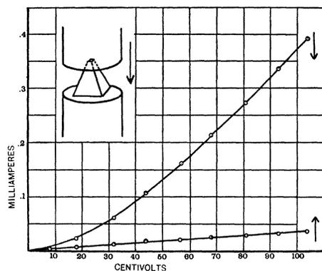
Fig. 1. — Current-voltage curves for anatase, with direct current.
