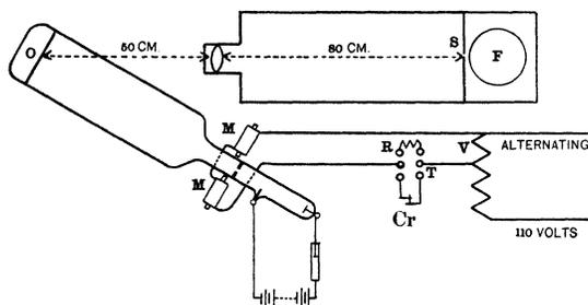
Fig. 6. Oscillographic apparatus.
