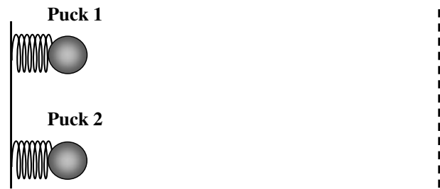
FIG. 22. Diagram of a low-friction table with two pucks launched by pushing them against two identical springs.
