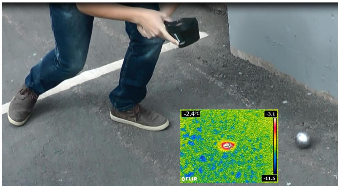
FIG. 2. A student using an IR camera to observe the point of impact immediately following dropping a steel ball onto asphalt, with an inset displaying the corresponding IR camera image of the impact surface.
