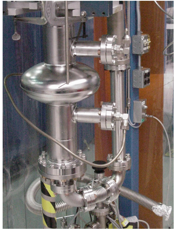
FIG. 2. (Color) CEBAF single-cell cavity with side-port loop couplers attached to the vertical test stand.
