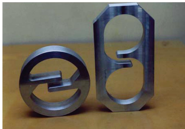
FIG. 15. (Color) Slices of the cylindrical and rectangular rf deflectors.
