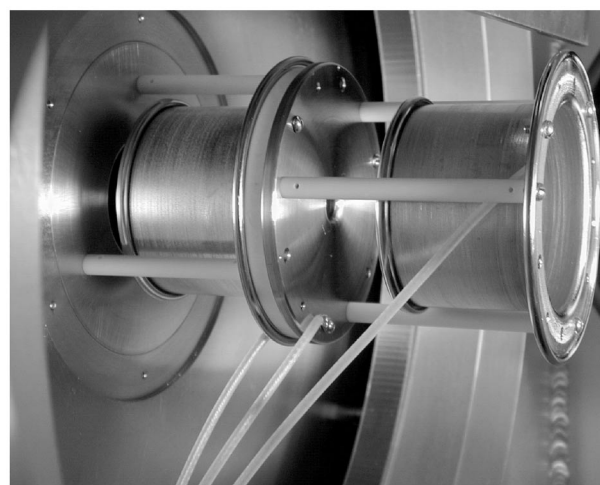
FIG. 10. Photograph of the NTX beam scraper system.
