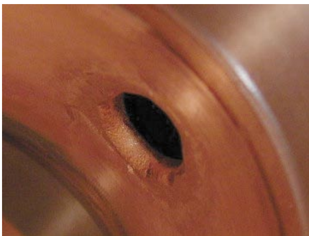
FIG. 22. (Color) A picture of the high-power coupling aperture of cavity 1 after the first high-power test. The aperture has been rounded in the direction of the magnetic field. The electric field has caused pitting to occur on either side of the aperture at right angles to the rounding.
