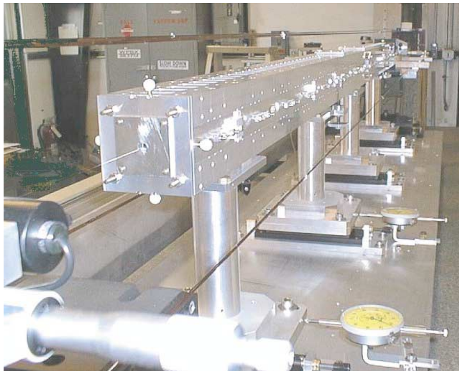
FIG. 6. (Color) Two segments of the VISA undulator mounted on the stretched wire testing stand. The wire may be seen passing down the axis of the undulator.
