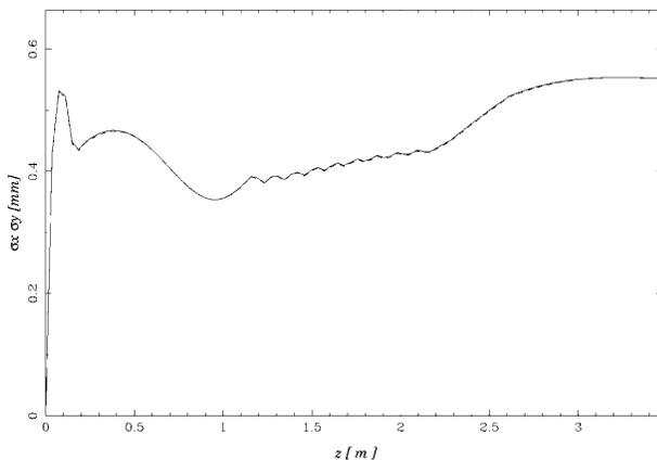
FIG. 5. Transverse beam size as a function of position along the beam line.
