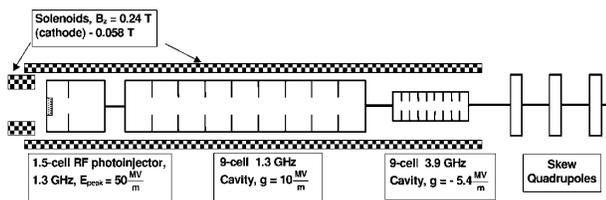
FIG. 1. Sketch of the electron beam source layout.
