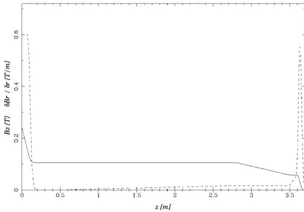
FIG. 4. Solenoid field strength  $B_z$  (solid line) and radial derivative  $dB_r/dr$  (dashed line) as a function of position along the beam line.
