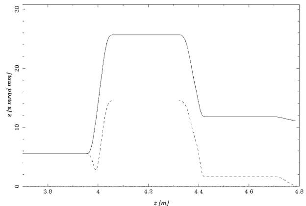
FIG. 6. Evolution of the horizontal (solid line) and vertical (dashed line) beam emittances in the skew quadrupole triplet.
