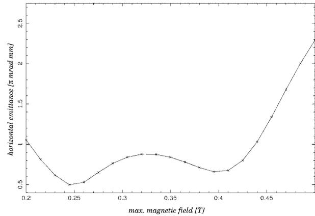
FIG. 2. Horizontal emittance obtained from ASTRA [6] simulations at the exit of the rf gun vs solenoid field at the cathode.
