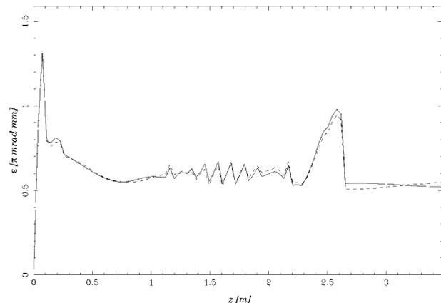
FIG. 3. Horizontal and vertical emittances obtained from ASTRA [6] simulations for the electron source up to position  $z$  just before the end of the solenoid.
