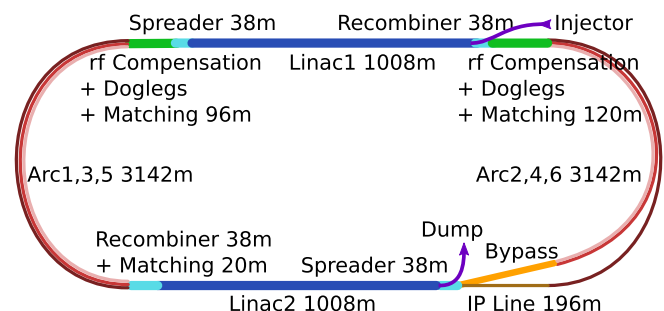
FIG. 1. Scheme of the LHeC electron facility.
