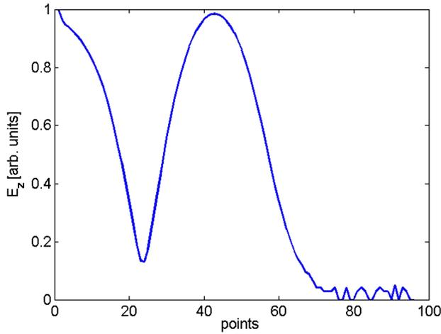
FIG. 9. Measured accelerating field profile after tuning.
