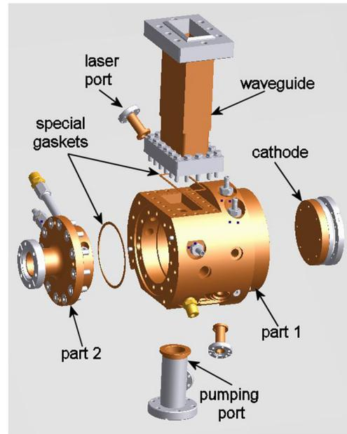
FIG. 6. Mechanical drawing of the gun: detail of the assembly procedure.
