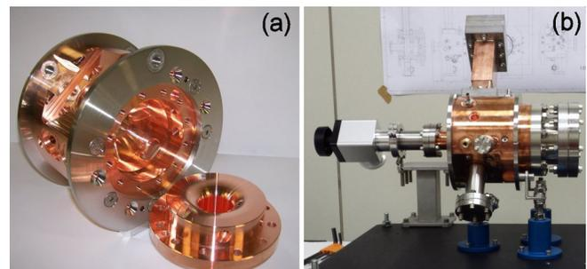
FIG. 8. Pictures of the gun before (a) and after the final assembly (b).
