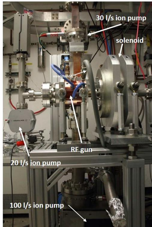
FIG. 12. Pictures of the rf gun installed in the Pegasus Laboratory at UCLA.
