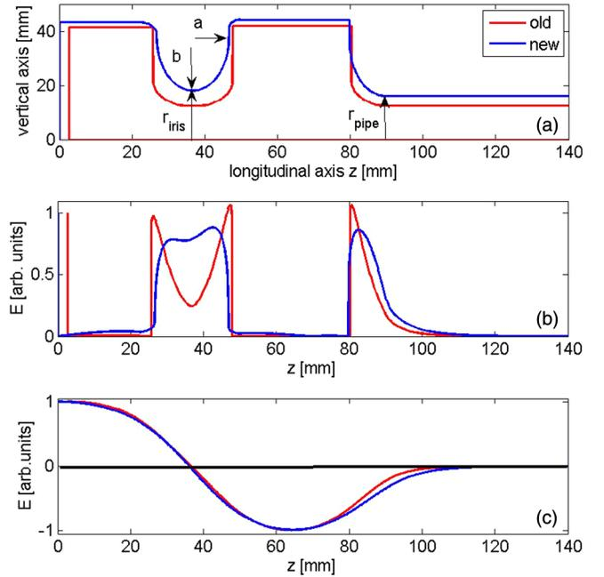
FIG. 1. (a) 2D profile (compared with the previous gun profile); (b) surface electric field normalized to the peak cathode field; (c) longitudinal electric field on axis.
