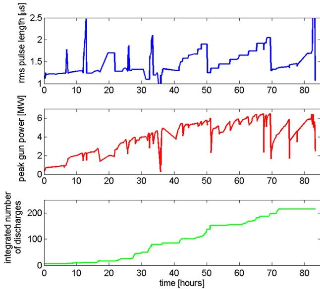
FIG. 13. Progress in power (measured from the gun probe), rms pulse length and integrated number of discharges during conditioning.
