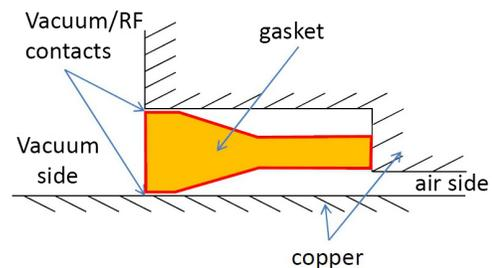
FIG. 7. Sketch of the transverse profile of the special vacuum/rf gasket used for gun clamping.
