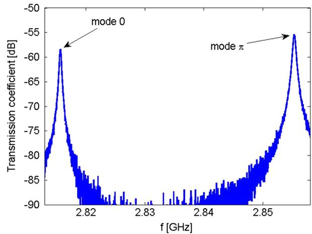
FIG. 11. Radio frequency gun resonant modes (measured in air at 60% relative humidity and 20°C).
