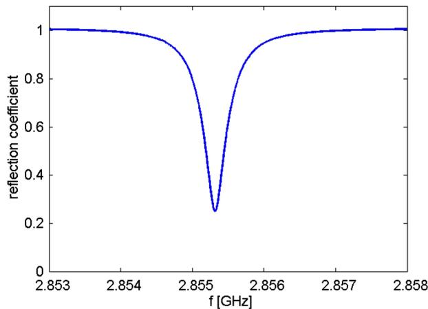
FIG. 10. Reflection coefficient at the input port (measured in air at 65% relative humidity and 20°C).
