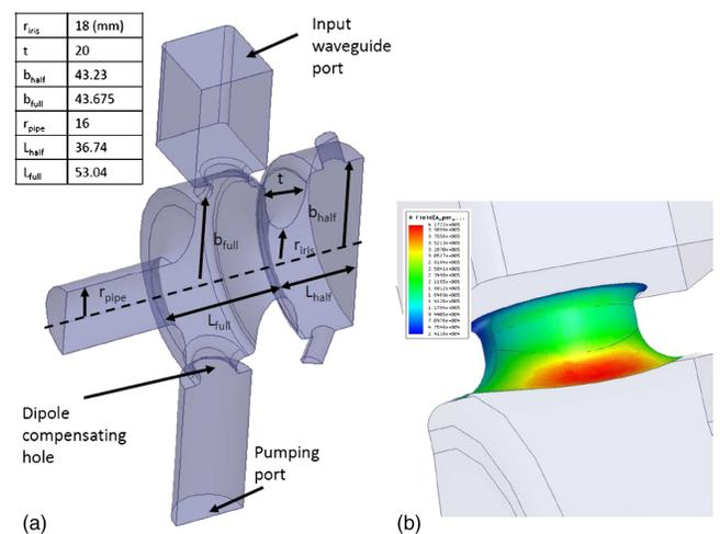
FIG. 2. (a) HFSS geometry of the rf gun; (b) detail of the surface peak magnetic field on the coupling hole at 120 MV/m on the cathode.
