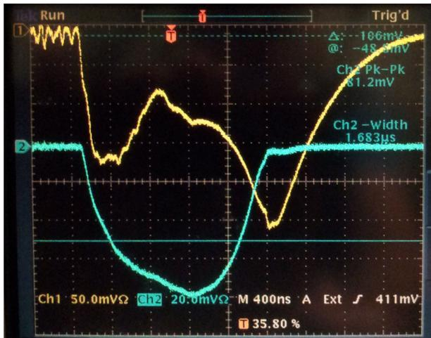
FIG. 14. Samples of monitoring signals during conditioning: cyan forward power, yellow reflected power.
