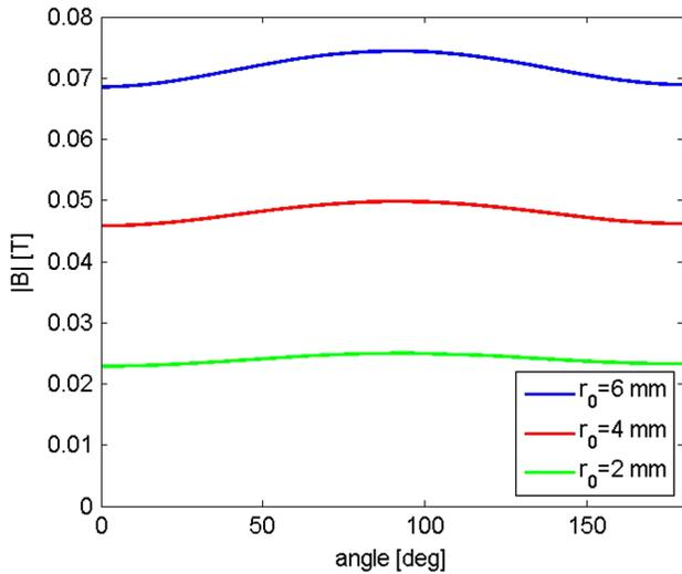
FIG. 17. Azimuthal magnetic field in the center of the full cell (referred to the case of a 120 MV/m accelerating field on the cathode) for three different circle radii.
