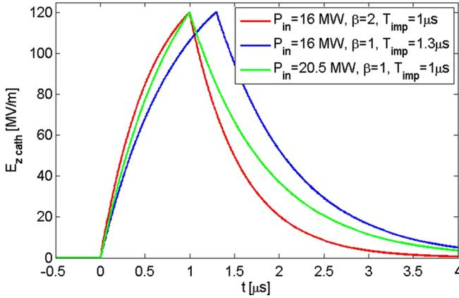
FIG. 3. Electric field on the cathode as a function of time in different cases.
