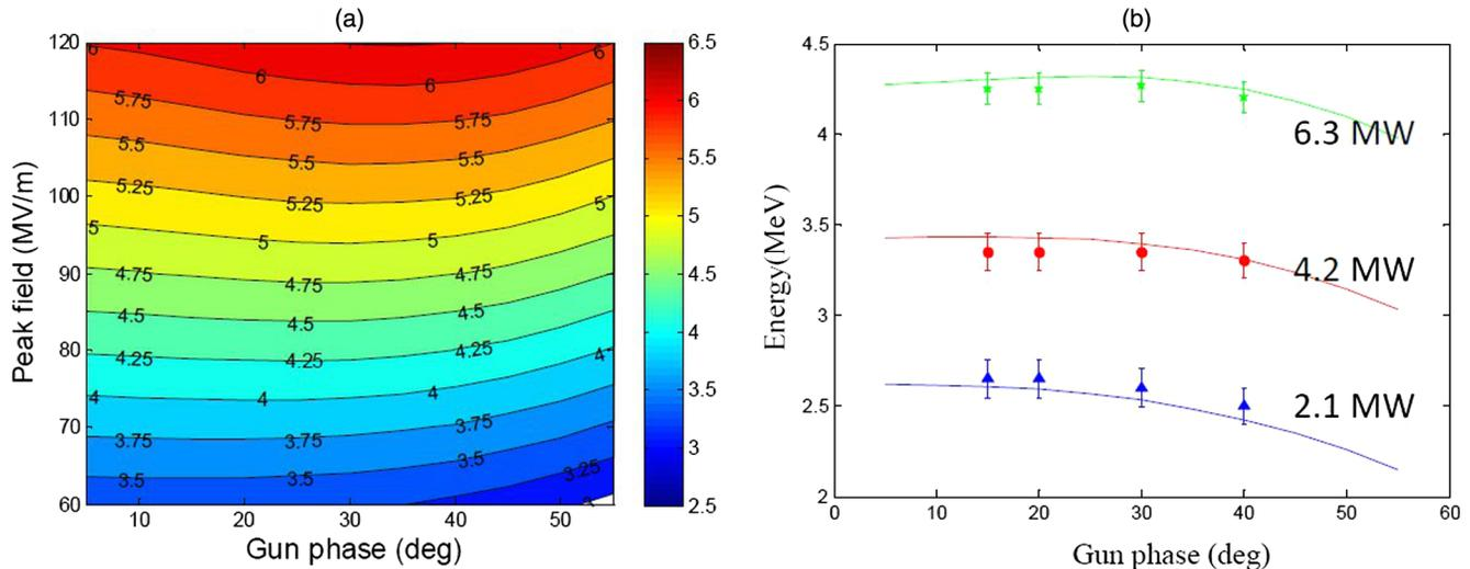
FIG. 16. (a) Theoretical maximum electron energy as a function of rf phase for different cathode peak field; (b) measured electron beam energy as a function of phase and for different power into the gun.
