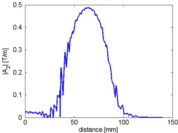
FIG. 18. Absolute value of the quadrupole gradient calculated using Eq. (A1) for  $r_0 = 8$  mm.
