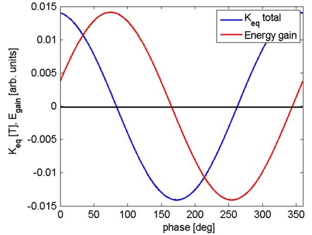
FIG. 4. Integrated quadrupole gradient as a function of the injection phase.
