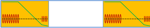
FIG. 1. An off-scale schematic of the proposed active-medium two-beam accelerator (AM-TBA) concept. The trigger train in each module generates Cherenkov radiation, which is amplified by the active medium—its amplitude is schematically described by the green line. As this amplification process saturates, the amplitude of the wake is virtually constant and it accelerates the trailing train of bunches.
