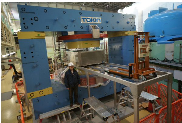
FIG. 4. The proof of principle system using a spectrometer magnet. An annealing oven is located between the magnet poles. A load lifter was used to set a core in the oven.
