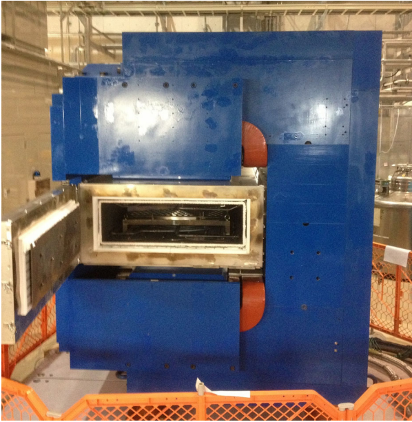
FIG. 11. The FT3L core production system using the Kappa magnet. The inner size of the oven is 1.1 m(W) \times 0.37 m(H) \times 1.4 m(L) to anneal the large size core up to 0.85 m diameter.
