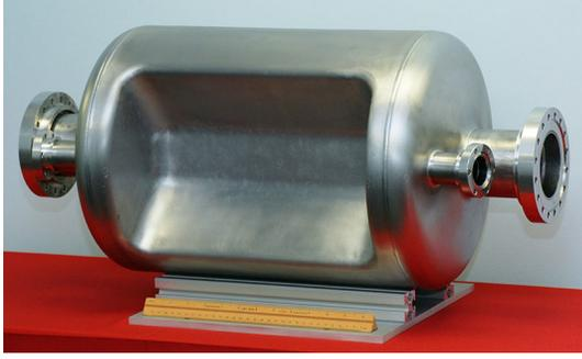
FIG. 4. Fabricated 400 MHz rf-dipole cavity.
