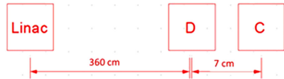
FIG. 5. Setup for the one-step correction. D is the position for velocity diagnostic and C is the position for the velocity correction.
